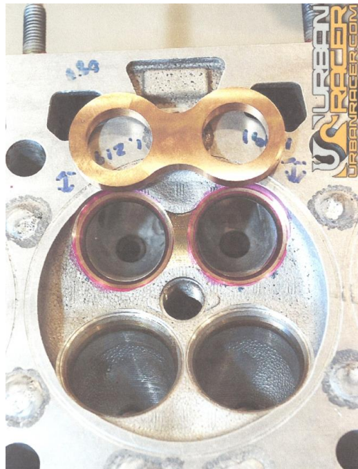
Figure 3. Combustion chamber of the GM Ecotec, as adapted to high boost drag racing. Features include no horizontal squish, dry deck and a one piece exhaust valve seat designed to maintain exhaust seat integrity at very high specific power levels.
